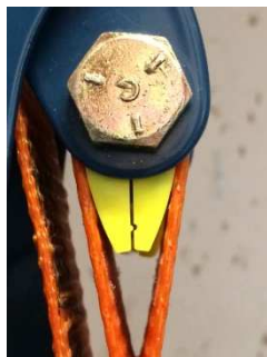
Display tightened up to the first mark. The pretensioning force applied is 750 daN.
